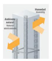
Rust contributes to microscopic porosity in steel, which increases its adherence to concrete and avoids structure slipping.
